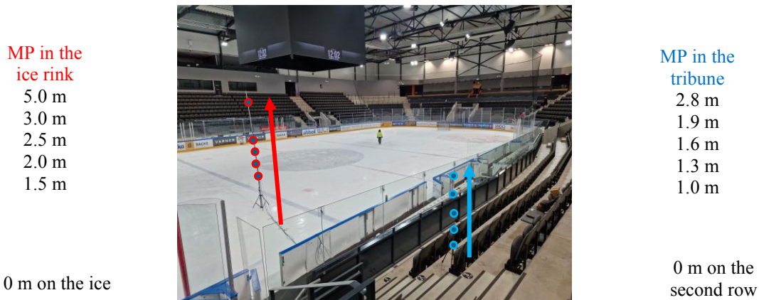
Figure 1: Measurements positions (MP) at the same time, five microphones in the ice rink and five microphone on the tribune.
