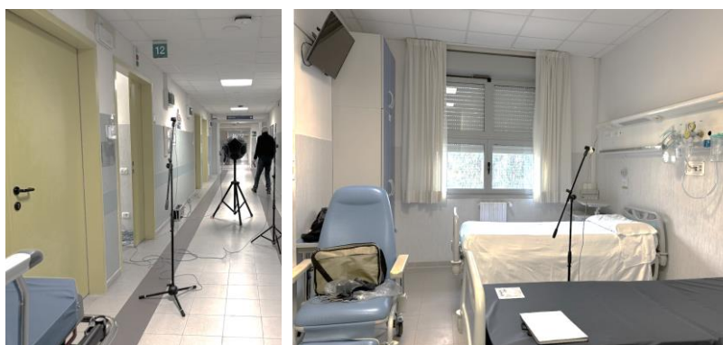
Figure 2: Example of one of the four case studies analysed: Endocrine Surgery Ward. Sound insulation measurements of the partition between the bedroom and the corridor (on the left), and between two adjacent bedrooms (on the right).
