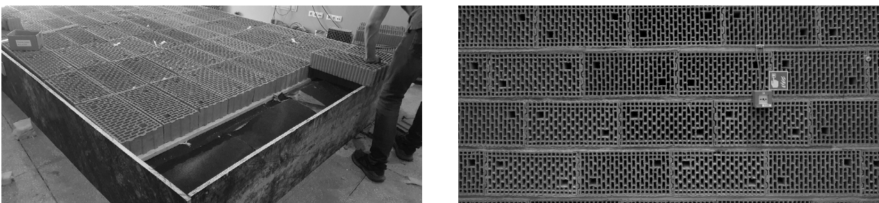
Figure 5: Brick cladding used on walls in all television studios (left: during ISO354 test, right: finished in hall)
