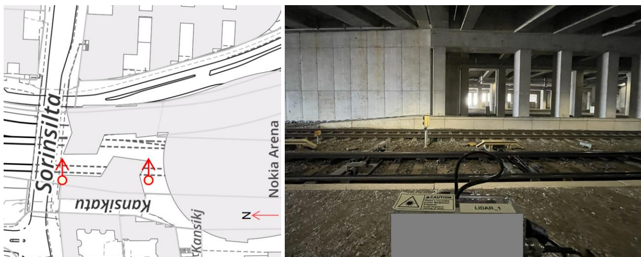
Figure 1: Locations of the lidar units in the tunnel (left) and the southern lidar unit's line of measurement (right).
