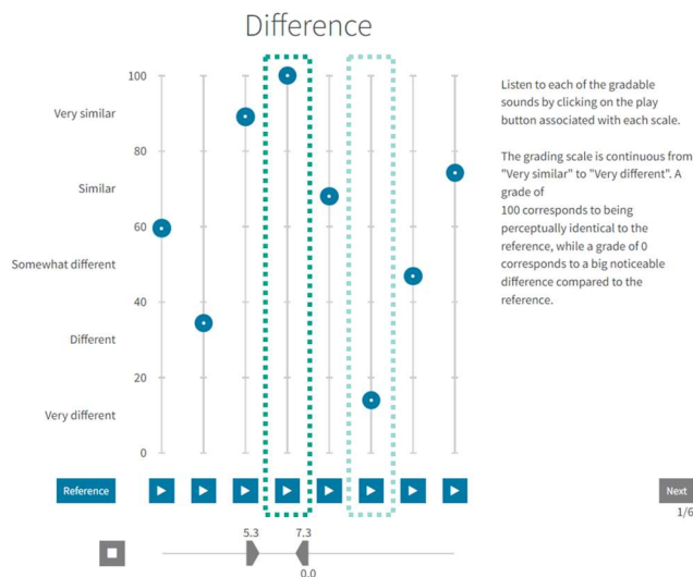
Figure 1: MUSHRA test interface in SenseLabOnline listening test software, showing the systems, scales, and description. The dark green dashed box marks the stimulus the assessor identified as the hidden reference, placed in the top, and the light green dashed box marks the anchor. The remaining systems (play buttons) hold a random order of the two Odeon simulations, the three Treble simulations and the Raven simulation (in the BRAS geometries).
