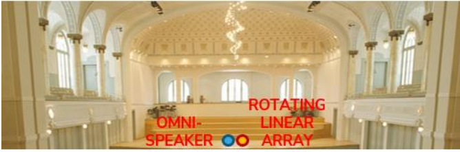
Figure 14. Arrangement of omnidirectional source and rotating linear array in the stage area of a concert hall.
