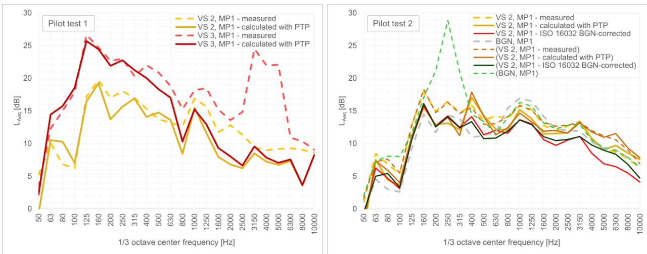
Figure 4: Ventilation noise levels in ventilation setting “VS 2” in microphone position MP1 – measurements and calculations according to the pilot test procedure (PTP) for pilot test 1 (on the left) and 2 (on the right). Brackets indicate repeated measurements.
