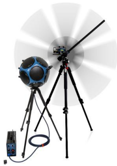
Figure 15. Co-located arrangement of omnidirectional source and rotating linear array.
