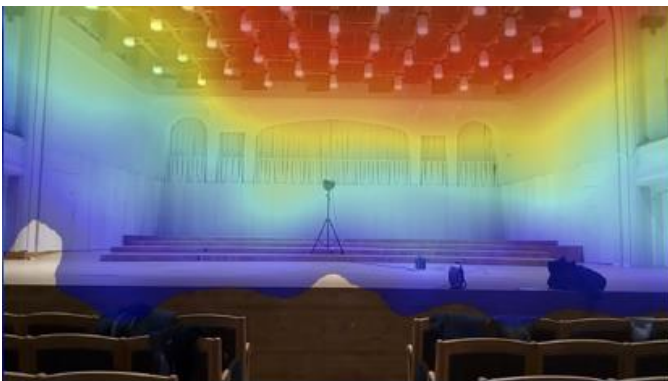
Figure 21. Critical reflections located at the point of observation. Selected frequency band is 250Hz – 3.1kHz at a dynamic range of 6dB.
