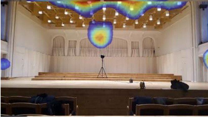
Figure 20. Primary reflections located at the point of observation. Selected frequency band is 250Hz – 3.1kHz at a dynamic range of 2dB.
