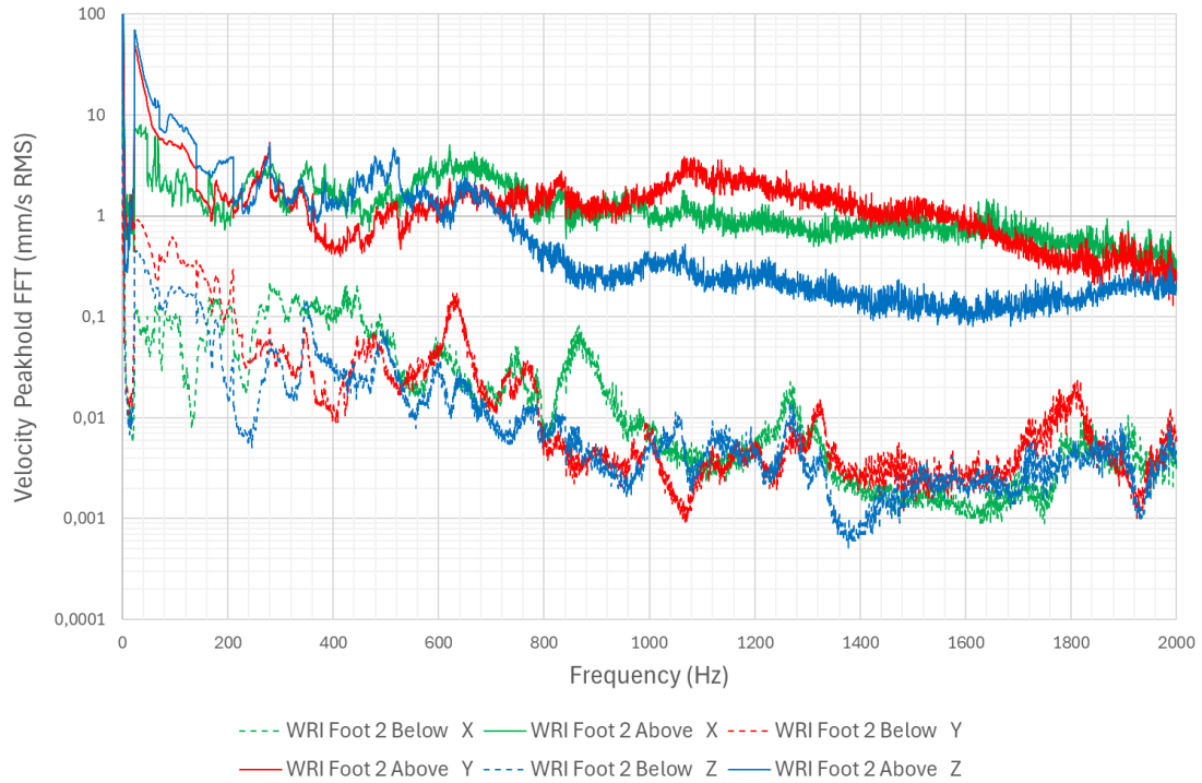
Figure 2. Vibration velocity peak-hold. Three directions – WRI. Sweep test from 2100 to 700 rpm.
